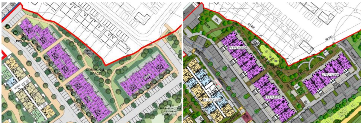
Figure 33 Layout of the northeast corner as submitted for the pre-application consultation request to the left and the current proposed layout for the northeast corner for the planning application to the right
